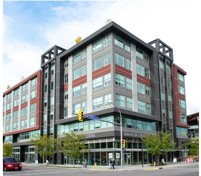
Figure 48 - Building corners on intersections should be distinguished, for example through structural elements and the use of glazing. Source: Central Okanagan Economic Development Commission. https://www.investkelowna.com/key-sectors/digital-tech/
